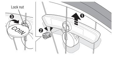
Place the nut into the reflector hole putting the spoke in between then tighten it securely using a coin.
