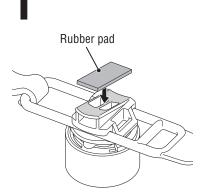
Attach securely in the mounting position.
