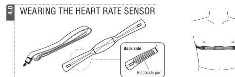
The Heart Rate Sensor is used to count your heartbeat and transmit the data to the MSC-HR10/20. **To wear the Heart Rate Sensor:**
