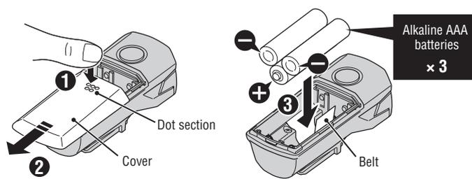
1. Slide the cover backward while pressing on the dot section (Fig.1 ①, ②).
