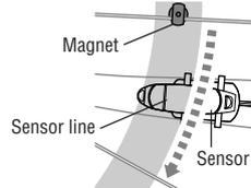
**B** The clearance between the sensor surface and the magnet must not exceed 3 mm.
